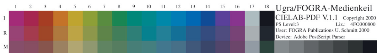
Fig. 4b: Ugra/Fogra media wedge CIELAB (available as TIFF, EPS and PDF Version, see glossary)
