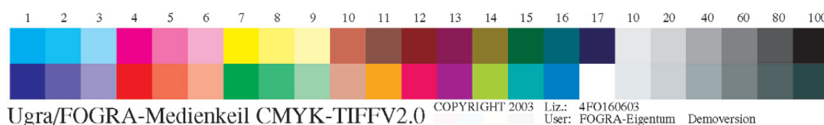
Fig. 4a: Ugra/Fogra media wedge CMYK (available as TIFF and EPS Version, see glossary)
